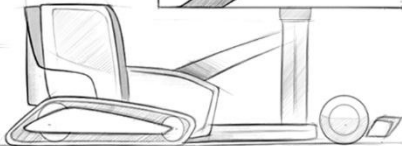
• caterpillar belt is used so that it can revolve on the spot
